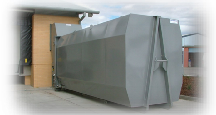
Single Auger Compactor ALDI Store
